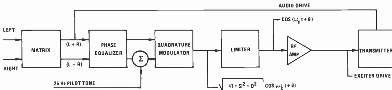
Note that the audio modulation sum information is unchanged from the monaural case and that a quadrature phase modulated RF drive is substituted for normal RF drive. The only other change is the presence of a Phase Equalizer to compensate for the differences in Amplitude/Phase relationships between the audio signal path and the RF path. This is necessary to maintain separation over a wide bandwidth.
